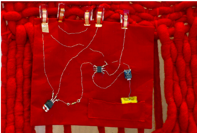
Textile electronic circuit. You can just clip it on and off.
